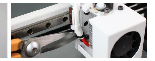
**4.** Disconnect the cable from the hotend pressing de connector.
