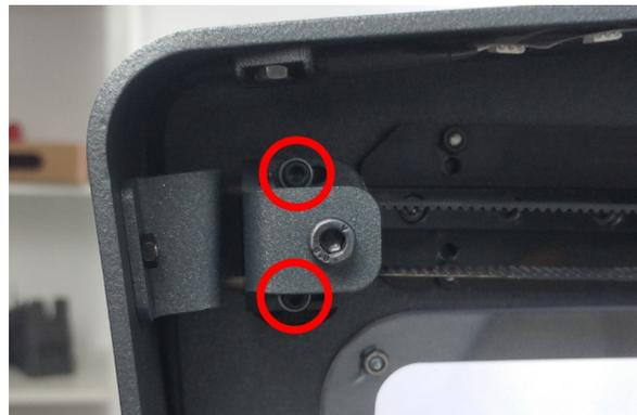
7. Adjust the screws on the side of the idler. Loosening them will decrease belt tension, tightening will increase. You still need to support the tool, as seen below.
