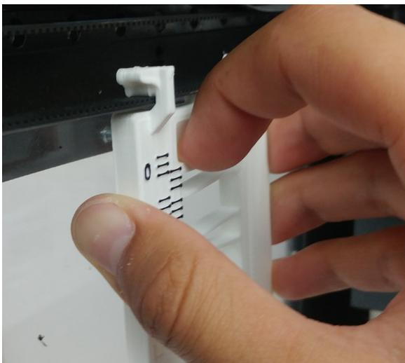
12. Let the device hang from the belt, without twisting. You can use a hand to stabilize it, but for reading you shouldn't touch it.
